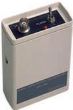
The NG-281/NG-282 noise generators are large bandwidth devices especially designed for application in all kinds of television installations, whether terrestrial, cable or satellite distribution. The frequency range of the NG-282 is from 950 to 2000 MHz, and the NG-281 from 5 to 1000 MHz.
